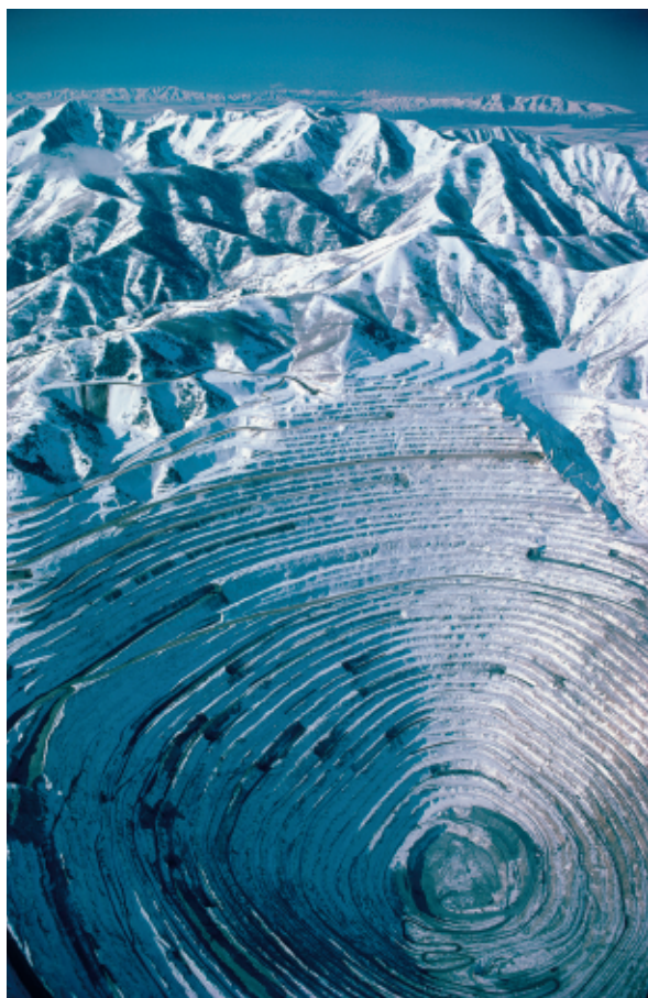
Figure 3 With a rim diameter of 4 km and a depth of almost 1 km, the Bingham Canyon Mine in Utah is the largest copper mine in the world.
