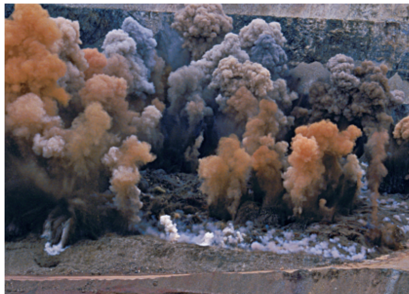
Figure 1 The surface of this gold mine in Nevada is being blasted to remove layers of rock.
